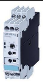
TIME RELAY, MULTI-FUNCTION 2 CHANGEOVER, 16 FUNCTIONS, 15 TIME SETTING RANGES AC 24/200... 240 V AND DC 24V, WITH LED, SCREW CONNECTION
