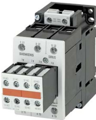
CONTACTOR, 3PH, 22 KW/400 V, 120 V AC, 60 HZ, 2NO+2NC,
