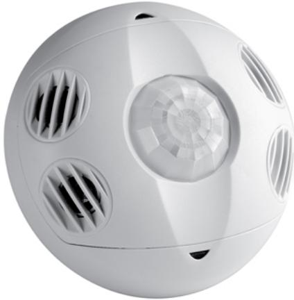
Occupancy Sensor, Ceiling Mounted, Multi-technology, 24VDC, 30mA power consumption, 2000 sq ft, 360 degree (major motion: PIR: 40' diameter; U/S:64'Lx32'W, minor motion: U/S: 45'Lx23'W), red LED=PIR, green LED=U/S auto adapting, walk-through, time delay 30s-30m, test mode (6s time delay for 15m with auto exit), connect gray wire for photocell ambient light hold-off, 360 degree harmonic wheel (rotatable), mounting height 8'-10', cUL/NOM listed, CEC Title 24 compliant. Color: true-white.
