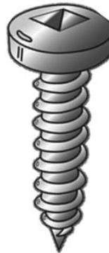
*Sheet Metal Screws (Self-Tapping Screws) are threaded fasteners with sharp threads to cut into materials such as sheet metal, plastic, or wood.*
