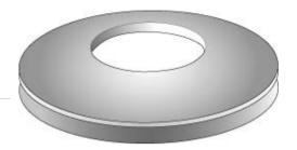
A slightly concave, metal-backed, rubber or neoprene washer that is typically placed on a fastener to prevent water from migrating into and through the fastener hole.
