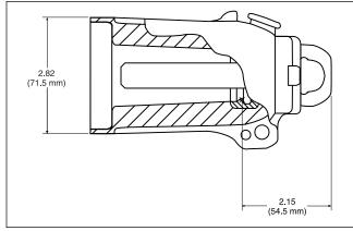
**Figure 3.**15 kV Insulated Protective Cap profile and stacking dimensions.
