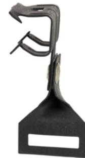
Side Mount Flange Clamp with Right Angle Strap Hanger, Fits 9/16 to 3/4" Flange, Suspends Strap up to 1" Wide, Spring Steel
