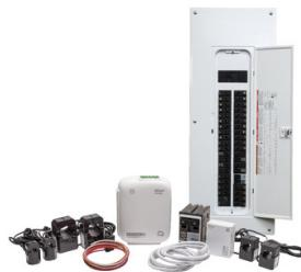
Load center, Homeline, 1 phase, 40 spaces, 80 circuits, 200A convertible main breaker, PoN, NEMA1, combo cover
