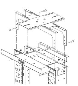
NFLRB assembles to NFR80J using M10 hex bolt, nut, and lockwasher provided with NFR80J.
