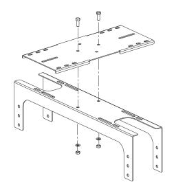
NFLRB Top Plate can be assembled perpendicular to Main Bracket to support parallel runs of ladder rack.
