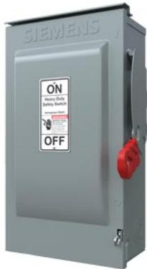
Siemens Low Voltage Circuit Protection Heavy Duty Safety Switch. 3-Pole 3-Fuse and solid neutral Fused in a type 3R enclosure (outdoor). Rated 600VAC (60A).
