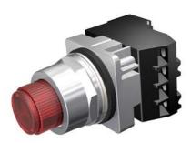
30mm Command/52, Chrome Finish Heavy Duty, Watertight/Oiltight Complete Metal Unit PTT / Illuminated Pushbutton Full Voltage, 120V AC/DC LED Lamp Extended Button Plastic Lens, Red 2 Position Momentary with 1 N.O. - 1 N.C. Heavy Duty Contacts, A600/P600 UL Listed, CSA Certified NEMA 1,3,3R,4,4X,12,13 & Automotive Standards
