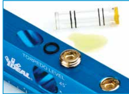
2. Remove O-ring and damaged vial
