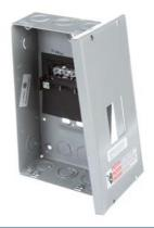
Siemens Energy Management Residential Specialty Load Centers: Small Circuit (2-10). Sub Brand: Load Centers Type: 1: Application: Residential: Voltage Rating: 120/240V Amperage Rating: 60A Phase: 1PH Load Regulation: 60A Wiring Configuration: 3w Bus Rating: 60A Interrupt Rating: 100000AIC. EQ LC 2S 4C ML 60A N1-S
