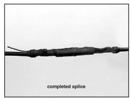
Note: In applications where the splice is regularly exposed to high levels of ultra-violet radiation (i.e. direct sunlight), wrap two half-lapped layers of Scotch<sup>™</sup> Super 33+ or Scotch<sup>™</sup> Super 88 vinyl tape over the re-jacketing tubes.
