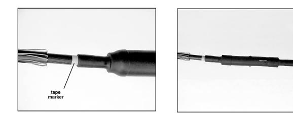
Note: Do not push the splice body towards the tape marker, as this may cause the end to roll under. If the end does roll under, DO NOT use sharp edged tools to pull it out as this could cut and damage the splice.
