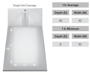
Meets Life Safety Code minimum illuminance of 0.1 fc and average illuminance of 1.0 fc. Assumes open space with no obstructions, mounting height of 7.5', ceiling height of 9' and reflectances of 80/50/20. Photometry files available on the Dual-Lite web site (www.dual-lite.com).
