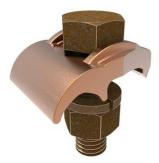
Mechanical Grounding Connector, Cable to 1/4" Thick Bar, 4 AWG (Sol)-2/0 AWG (Str), 3/8" Stud.
