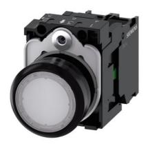
Illuminated pushbutton, 22 mm, round, plastic, white, pushbutton, flat, momentary contact type, with holder, 1 NO, LED module with integrated LED 24 V AC/DC, screw terminal
