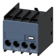
auxiliary switch, on the front, 1 NO + 1 NC, 73/74, 81/82, current path: 1 NO, 1 NC, cable entry from below, screw terminal, for contactors 3RT2 and contactor relays 3RH2
