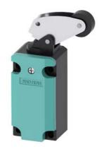
Position switch Metal enclosure 40 mm according to EN 50041 Device connection 1x (M20 x 1.5) 1 NO/1 NC quick action contacts Angular roller lever, metal lever and plastic roller 22 mm
