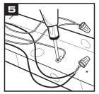
With power off, make power supply connections as shown. Attach ground wire to green ground screw, connect power supply.
