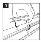
Squeeze channel at markers shown to remove channel cover.
