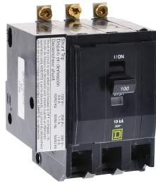
Mini circuit breaker, QO, 100A, 3 pole, 120/240VAC, 10kA, bolt on, AC shunt, ring
