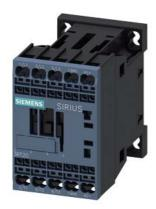
power contactor, AC-3e/AC-3, 7 A, 3 kW / 400 V, 3-pole, 24 V DC, auxiliary contacts: 1 NO, spring-loaded terminal, size: S00  $\,$
