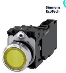
Illuminated pushbutton, 22 mm, round, metal, shiny, yellow, pushbutton, flat, momentary contact type, with holder, 1 NO+1 NC, LED module with integrated LED 24 V AC/DC, screw terminal
