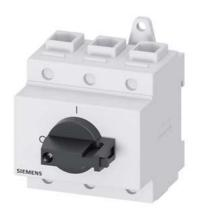
SENTRON, Switch disconnector 3LD, main switch, 3-pole, lu: 100 A, Operating power / at AC-23 A at 400 V: 37 kW, installation in distribution boards, knoboperated mechanism, black, handle direct at the switch
