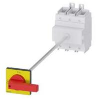
SENTRON, Switch disconnector 3LD, emergency switching-off switch, 3- pole, lu: 160 A, operating power / at AC-23 A 400 V: 75 kW, floor mounting with door coupling, knob-operated mechanism, red/yellow, 4-hole mounting of the handle
