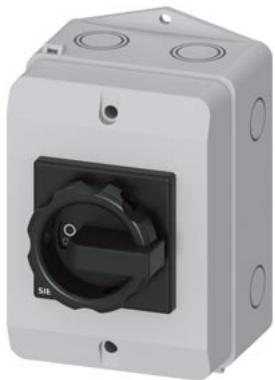
SENTRON, Switch disconnector 3LD, main switch, 3-pole, I<sub>u</sub>: 32 A, Operating power / at AC-23 A at 400 V: 11.5 kW, molded-plastic encapsulation for inch cable gland, 2 NO, rotary operating mechanism, black
