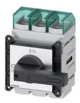
SENTRON 3LD5 switch disconnector UL, main switch, 3-pole, approved according to UL 489, UL 60947-4-1 and IEC 60947-3, UL: 150 A, SCCR 50 kA at 480 V AC, operational power @ 480 V AC 3-phase: 100 hp, IEC: 160 A, operational power at AC-23 A at 400 V: 75 kW, front-mounted: rotary operating mechanism, black, 4-hole mounting of the handle, including terminal covers for the infeed side infeed side
