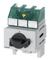
SENTRON 3LD5 switch disconnector UL, main switch, 3-pole, approved according to UL 489, UL 60947-4-1 and IEC 60947-3, UL: 30 A, SCCR 50 kA at 480 V AC, operational power @ 480 V AC 3-phase: 20 hp, IEC: 32 A, operational power at AC-23 A at 400 V: 15 kW, floor mounting with direct operating mechanism, black, including terminal covers for the infeed side for the infeed side
