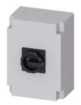
SENTRON, Switch disconnector 3LD, main switch, 6-pole, lu: 63 A, Operating power / at AC-23 A at 400 V: 22 kW, molded-plastic encapsulation for metric screw connection, 1 NC, 1 NO, rotary operating mechanism, black
