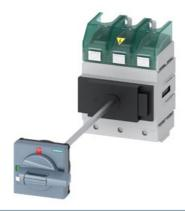
SENTRON 3LD5 switch disconnector UL, main switch, 3-pole, approved according to UL 489, UL 60947-4-1 and IEC 60947-3, UL: 100 A, SCCR 65 kA at 480 V AC, operational power @ 480 V AC 3-phase: 60 hp, IEC: 100 A, operational power at AC-23 A at 400 V: 45 kW, floor mounting with door coupling, defeatable rotary operating mechanism, standard, 4-hole mounting of the handle, without tolerance compensation, including terminal covers for the infeed side for the infeed side
