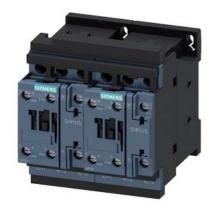
reversing contactor assembly, AC-3e/AC-3, 32 A, 15 kW / 400 V, 3-pole, 24 V AC, 50/60 Hz, screw terminal, electrical and mechanical interlock, auxiliary contacts: 2 x 1 NO
