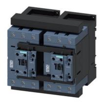
reversing contactor assembly, AC-3e/AC-3, 110 A, 55 kW / 400 V, 3-pole, 110 V AC, 50/60 Hz, screw terminal, electrical and mechanical interlock, auxiliary contacts: 2 x 1 NO
