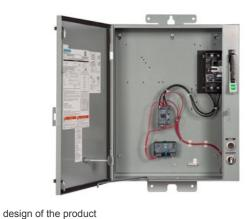
Pump control panel, NEMA Size 1, Three phase full voltage, 25A motor circuit protector, Solid-state overload relay, OLR amp range 5.5-22A, 480 V AC 60Hz coil, HOA selector switch, Start push button, Enclosure NEMA type 3R, Weather proof outdoor use, Standards: UL 60947-1, Certifications: cULus, Listed Service Entrance Equip
