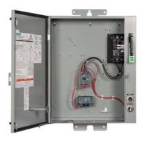
Pump control panel, NEMA Size 1, Three phase full voltage, 3A motor circuit protector, Solid-state overload relay, OLR amp range 0.75-3.4A, 480 V AC 60Hz coil, HOA selector switch, Start push button, Enclosure NEMA type 3R, Weather proof outdoor use, Standards: UL 60947-1, Certifications: cULus, Listed Service Entrance Equip
