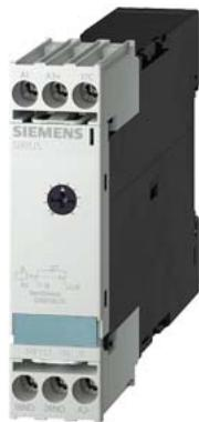
Timing relay, electronic Phased-out product !!! For further information, please contact our sales department with star-delta (wye-delta) function 1 NO contact, delayed 1 NO contact, instantaneous 1 time range 1...20 s 24 V AC/DC and 200...240 V AC at 50/60 Hz AC screw terminal
