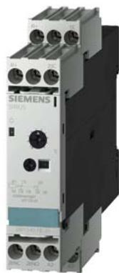
Timing relay, electronic Phased-out product !!! For further information, please contact our sales department OFF delay 2 change-over contacts, without auxiliary voltage 9 time ranges, 0.05 s...600 s 100...127 V AC/DC with LED, Screw terminal
