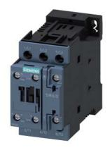
power contactor, AC-3e/AC-3, 32 A, 15 kW / 400 V, 3-pole, 48 V DC, auxiliary contacts: 1 NO + 1 NC, screw terminal, size: S0  $\,$
