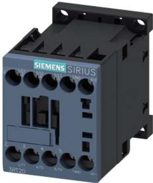
power contactor, AC-3e/AC-3, 9 A, 4 kW / 400 V, 3-pole, 24 V DC, auxiliary contacts: 1 NO, screw terminal, size: S00, upright mounting position
