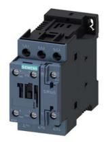
power contactor, AC-3e/AC-3, 12 A,  $5.5\,kW$  / 400 V, 3-pole, 200-280 V AC/DC, 50/60 Hz, with integrated varistor, auxiliary contacts: 1 NO + 1 NC, screw terminal, size: S0
