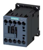
power contactor, AC-3e/AC-3, 7 A, 3 kW / 400 V, 3-pole, 24 V DC, auxiliary contacts: 1 NC, screw terminal, size: S00, communication-capable
