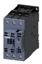
power contactor, AC-3e/AC-3, 41 A, 18.5 kW / 400 V, 3-pole, 24 V DC, 0.8-1.2\* Us, with integrated varistor, auxiliary contacts: 1 NO + 1 NC, main circuit: screw terminal, control and auxiliary circuit: spring-loaded terminal, frame size: S2, suitable for PLC outputs
