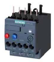
Overload relay 0.45...0.63 A Thermal For motor protection Size S00, Class 10 Contactor mounting Main circuit: Screw Auxiliary circuit: Screw Manual-Automatic-Reset
