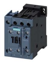
power contactor, AC-3, 25 A, 11 kW / 400 V, 4-pole, 230 V DC, main contacts: 2 NO + 2 NC, auxiliary contacts: 1 NO + 1 NC, screw terminal, size: S0
