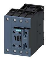
power contactor, AC-3, 35 A, 18.5 kW / 400 V, 4-pole, 175-280 V AC/DC, 50/60 Hz, with integrated varistor, main contacts: 2 NO + 2 NC, auxiliary contacts: 1 NO + 1 NC, screw terminal, size: S2
