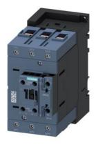
power contactor, AC-3e/AC-3, 110 A, 55 kW / 400 V, 3-pole, 175-280 V AC/DC, 50/60 Hz, with integrated varistor, auxiliary contacts: 1 NO + 1 NC, screw terminal, size: S3
