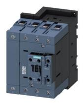
power contactor, AC-3, 65 A, 30 kW / 400 V, 4-pole, 110 V AC, 50 Hz / 120 V, 60 Hz, main contacts: 2 NO + 2 NC, auxiliary contacts: 1 NO + 1 NC, screw terminal, size: S3
