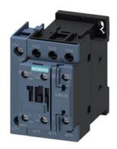
contactor AC-1, 40 A, 400 V / 40 °C, 4-pole, 220 V AC, 50 Hz / 240 V, 60 Hz, auxiliary contacts: 1 NO + 1 NC, screw terminal, size: S0
