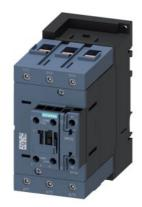
power contactor, AC-3e/AC-3, 80 A, 37 kW / 400 V, 3-pole, 208 V AC, 50/60 Hz, auxiliary contacts: 1 NO + 1 NC, screw terminal, size: S3  $\,$
