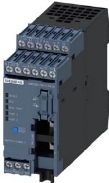
basic device SIMOCODE pro V PN GP , Ethernet/PROFINET IO, PN system redundancy, OPC UA server, web server, transfer rate 100 Mbps, 2 x bus connection via RJ45, 4 I/3 O freely configurable, Us: 24 V DC, input for thermistor connection monostable relay outputs, expandable by 1 expansion module(DM, TM, EM)
