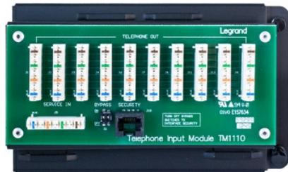
This telephone module is designed to distribute up to four incoming telephone lines (110 IDC Punchdown) to 10 locations, ensuring efficient and organized phone connectivity. It features a mar-resistant wall plate for durability and includes an RJ31X line seizure port for seamless security system integration. The module also comes with a mounting bracket for easy installation and is UL listed for safety and reliability.
